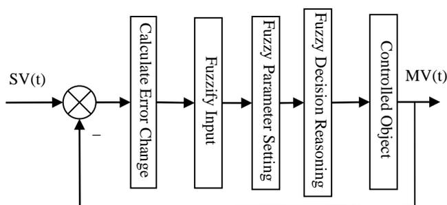
Figure 6. Fuzzy Control System Block Diagram
