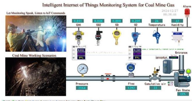
Figure 12. The Main Screen of the Intelligent IoT Monitoring System for Coal Mine Gas Using the Fuzzy-PID Algorithm.
