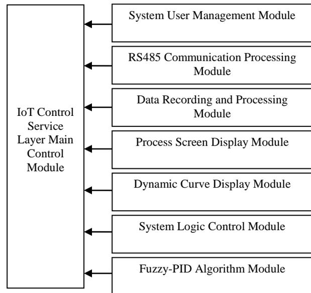
Figure 4. Function Module Diagram of the Control Service Layer in the IoT Monitoring System
