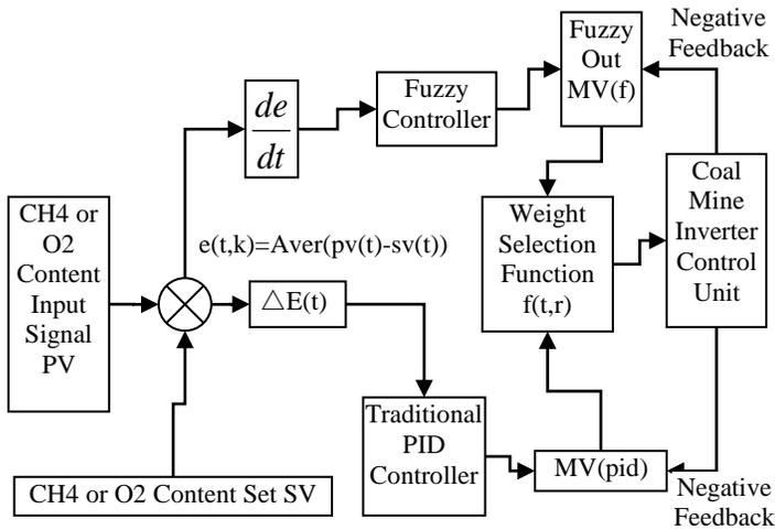
Figure 7. Coal Mine Gas Intelligent IoT Fuzzy-PID Control Schematic
