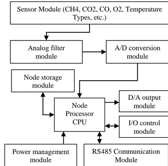
Figure 2. Functional Block Diagram of the Hardware Composition of IoT Sensor Nodes for Coal Mine Gas Monitoring
