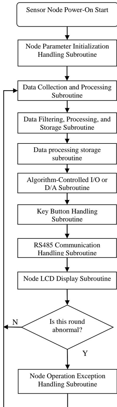
Figure 3. Flowchart of the Microcontroller Software Design for Sensor Nodes
