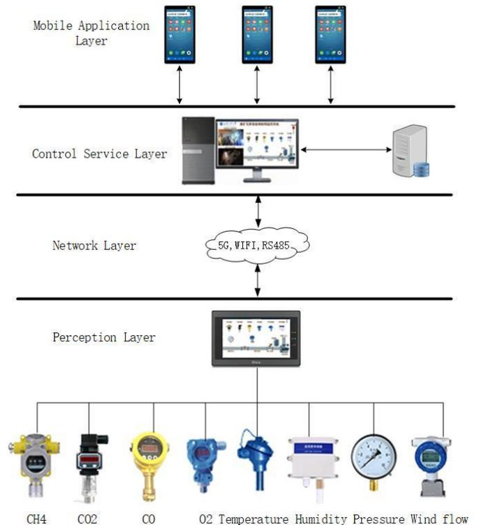
Figure 1. The Overall Architecture Diagram of the Intelligent IoT Monitoring System for Coal Mine Gas
