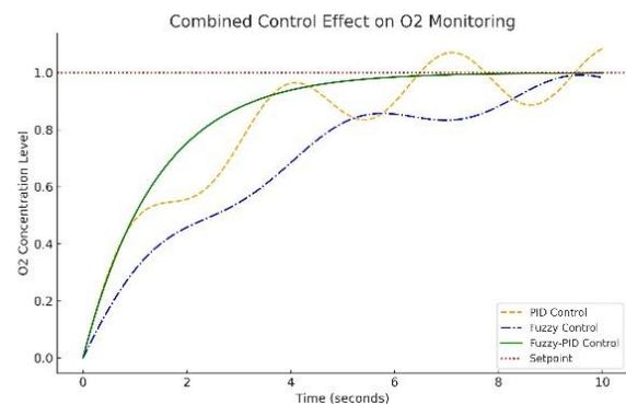
Figure 11. Comparative Experimental Control Effect Curve of the Three Algorithms.
