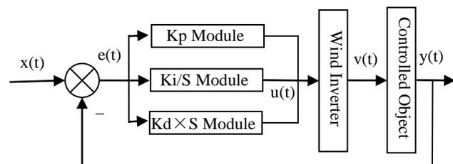
Figure 5. Traditional PID Control Process for Ventilation Variable Frequency Drives in Coal Mine Gas IoT
