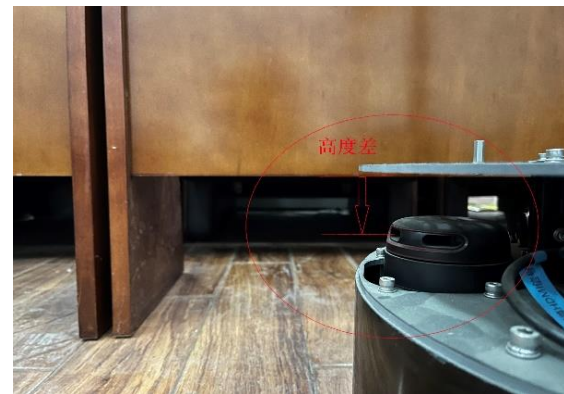
Figure 10. Installation height of LiDAR
