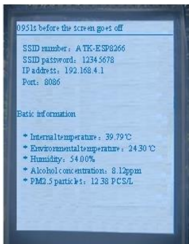
Figure 8. Wireless transmission interface
