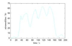
Figure 4. Soft threshold method airspeed denoising curve diagram.
