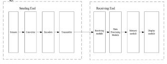
Figure 1. Overview of telemetry data processing structure.
