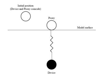
Figure 7. Mass-spring-damper Model
