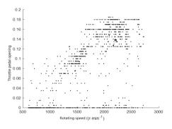
Figure 14. The relationship between driving speed and accelerator pedal
