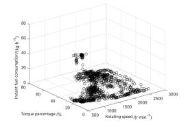
Figure 15. Instantaneous fuel consumption off for driving time and speed
