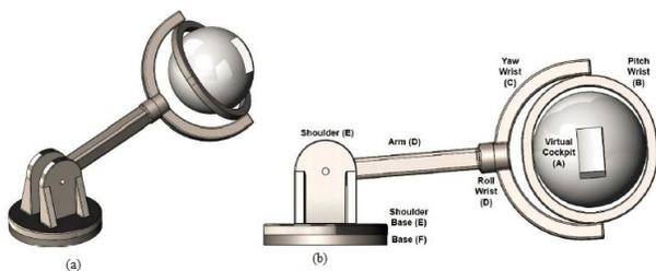
Figure 4. Simulator Isometric view (a) Labeled components (b)
