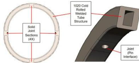
Figure 5. Pitch wrist cross section and structure
