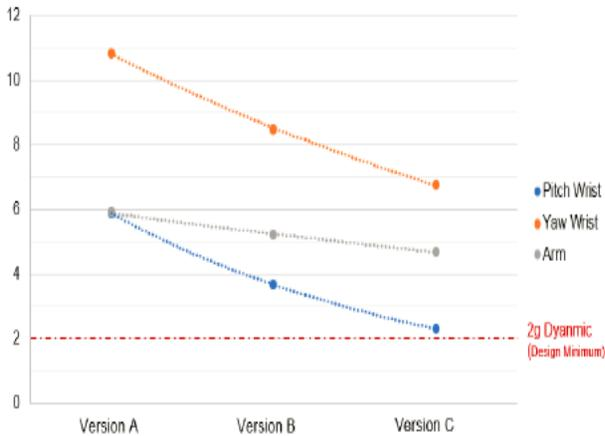
Figure 12. Gravity Loading Minimum Factor of Safety
