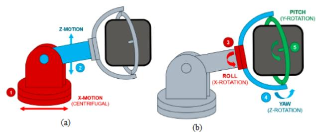
Figure 2. (a) Shoulder and arm function (simulated translational motion),
