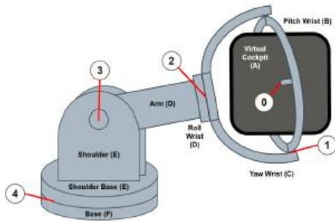
Figure 3. Robot Components (A-F) Robot Joints (0-4)
