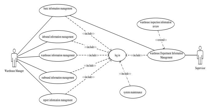
Figure 2. Use case diagram of intelligent warehouse management system.
