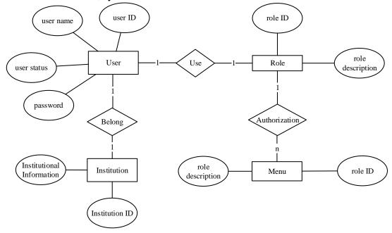
Figure 3. System E-R diagram.
