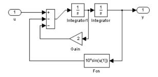
Figure 2. Simulink Block Diagram of Mechanical Arm
