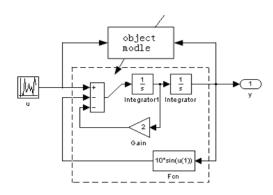
Figure 4. Neural Network Training Block Diagram of the Manipulator
