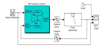
Figure 6. Simulation of Network Closed-Loop Control System based on Predictive Neural
