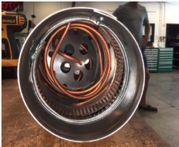
Figure 2. The heat exchanger prototype
