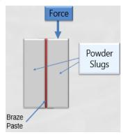
Figure 2. Tensile Testing Illustration
