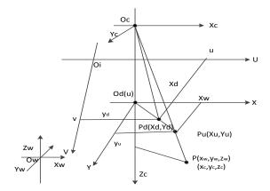
Figure 7. Camera distortion model diagram
