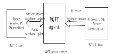
Figure 3. Figure 3 MQTT protocol communication model
