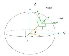
Figure 1. The local horizontal coordinate system and the geocentric coordinate system
