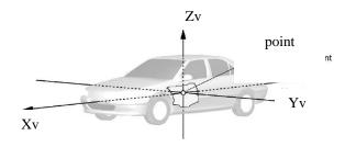
Figure 2. Car body coordinate system
