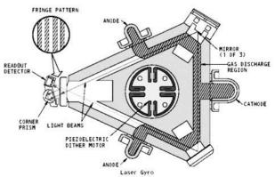
Figure 4. The principle of laser gyroscope works
