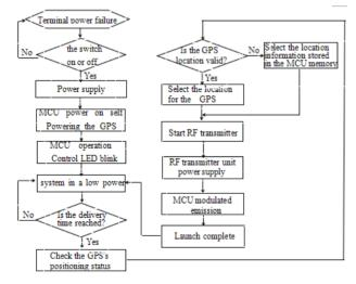
Figure 3. The process of micro-controller(MCU) active help terminal
