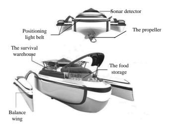
Figure 1. Intelligent Search and Rescue Device Structure Chart
