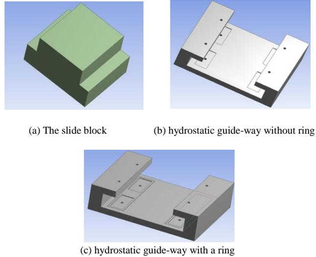
(a) The slide block (b) hydrostatic guide-way without ring
