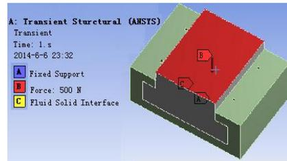
Figure 12. The edge condition of hydrostatic guide-way entity domain
