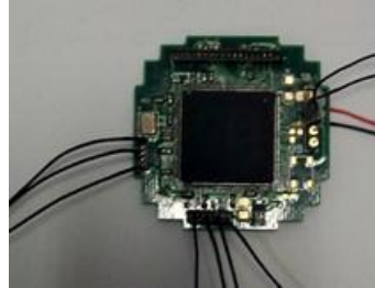
Figure 8. The frequency measurement module
