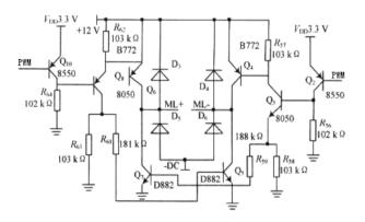
Figure 2. Motor drive circuit
