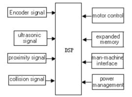
Figure 1. Structure diagram of control system
