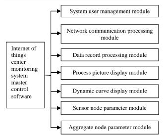
Figure 5. Module structure diagram of the IOT center computer monitor system software
