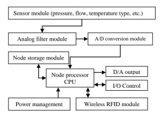
Figure 2. Hardware components theory block diagram of the fuel pump sensor instrument node
