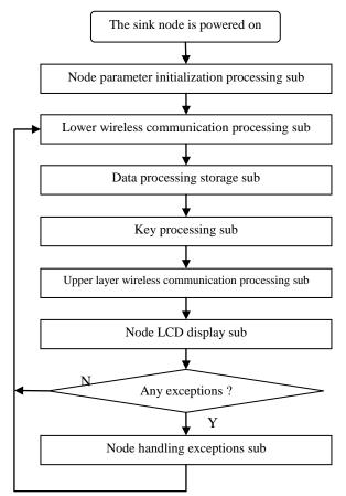
Figure 4. MCU control program flow chart of the IOT aggregation instrument node
