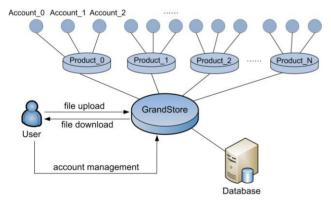
Figure 2. The architecture of GrandStore system.
