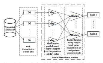
Figure 6. Framework of parallel algorithm mining association rules
