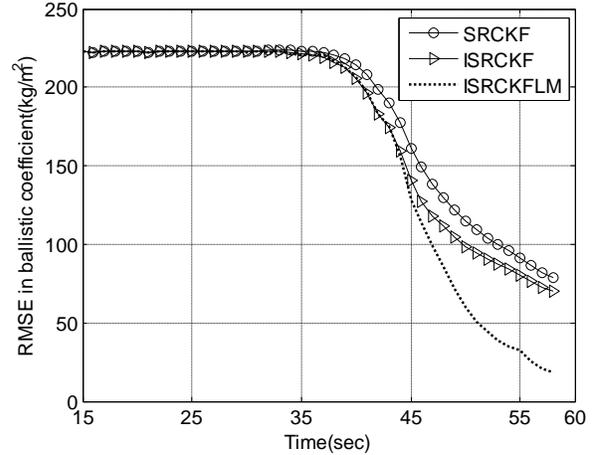
Figure 3. RMSEs in ballistic coefficient for various filters
