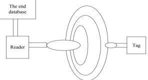
Figure.1 RFID system
